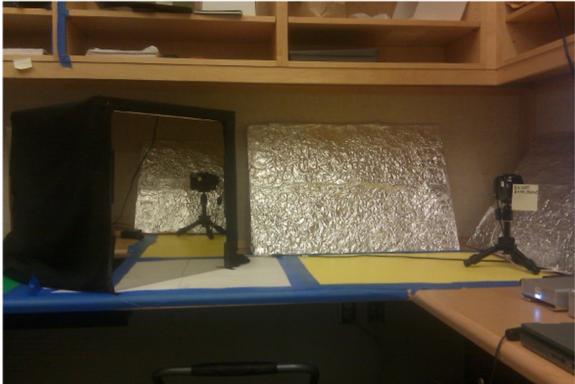
Figure 3. Photographic set up. Seen to the right is the FAR camera, also visible in the reflection in the mirror. Behind the mirror lies the CLOSE camera. The aluminum panels are present to provide additional illumination.
