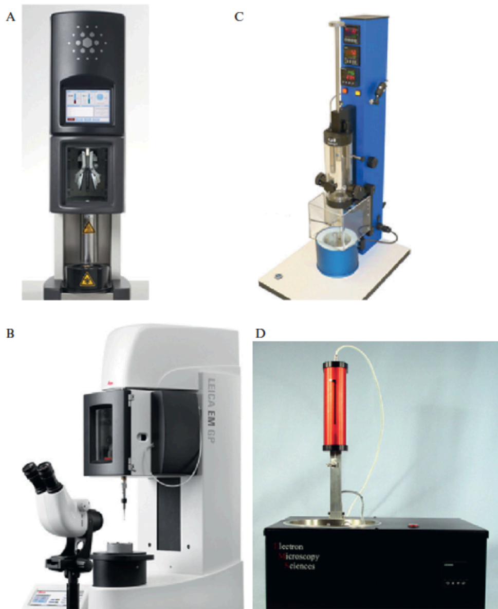
Figure 3.8. Variety of automated plunge freezers. (A) Vitrobot Mark IV, image courtesy of FEI, Inc., Hillsboro, OR, USA. (B) Leica EM GP, image courtesy of Leica Microsystems, Inc., Vienna, Austria. (C) Cryoplunge3, image courtesy of Gatan, Inc., Pleasanton, CA. (D) EMS-002 Rapid Immersion Freezer, image courtesy of Electron Microscopy Sciences, Hatfield, PA, USA.
