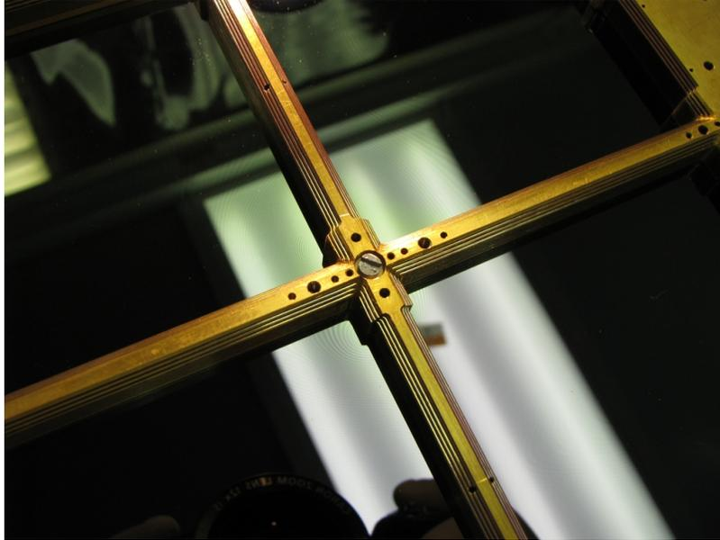
Figure 2.9: A close-up image of the illumination side of the focal plane unit, superconducting niobium center spacer screw and corrugated detector windows. Newton's rings are barely visible in several of the dark detector windows. They are created by small variations in the spacing between the antireflection and detector tiles.
