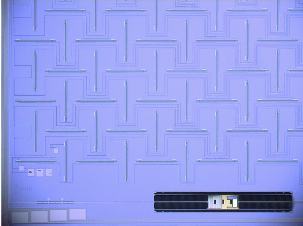
Figure 2.11: A micrograph (100x magnification) of a portion of a focal plane pixel, including the slot antenna, microstrip line and detector island.
