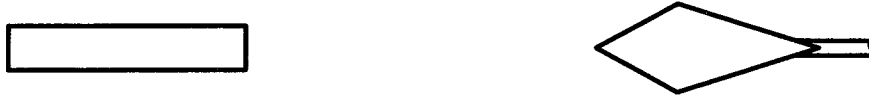
Figure 2.11. Two of the five shock generator geometries considered: a rectangular plate and a double-wedge.
