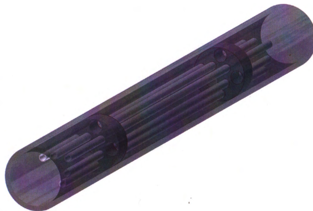
Figure 5.9: The structure of a Raman furnace, including ceramic rods, stainless flanges, and quartz tube
