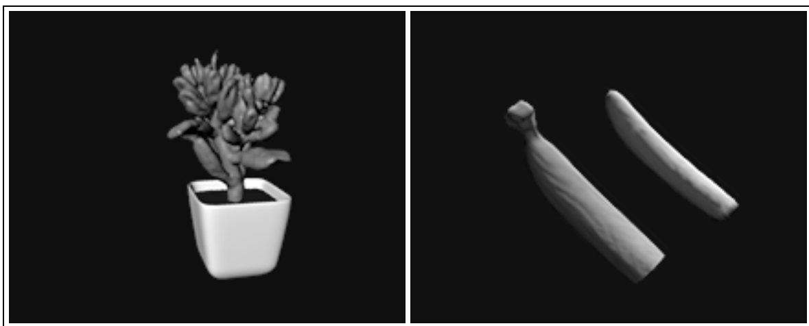
Figure 5.10: Geometric models extracted from volume data collected. A model of a jade plant is on the left. The model on the right is of banana skin and meat displayed separately. The banana model is cut off at the bottom because the real banana extended out of the uniform region of the MR coil. \square
