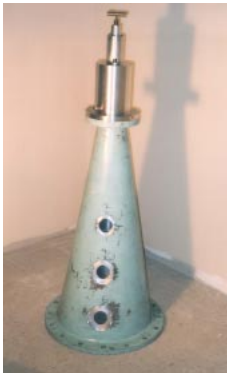
Figure 2.12: Photograph showing the cone with circular window apertures and extension installed.
