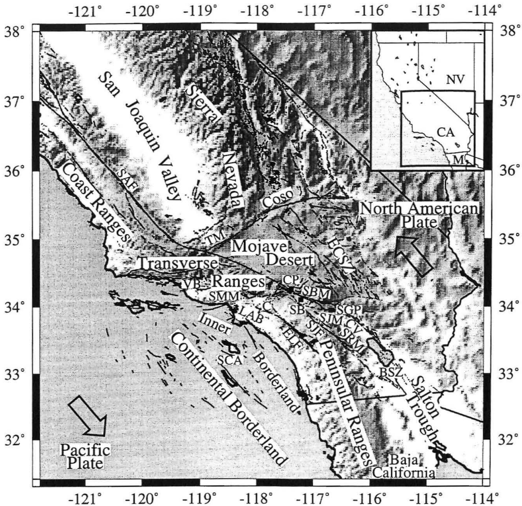
Figure 2.1 Tectonic and physiographic provinces of southern California in study area. Mapped surface traces of faults (Jennings, 1975) shown as thin black lines. The arrows show the approximate relative motion of the Pacific and North American plates. BSZ - Brawley Seismic Zone; C - Chino-Puente Hills; CA - state of California; CP - Cajon Pass; CV - Coachella Valley; ECSZ - Eastern California Shear Zone; LAB - Los Angeles Basin; NV - state of Nevada; M - Mexico; SB - San Bernadino (city); SBM - San Bernadino Mountains; SCA - Santa Catalina Island; SGP - San Gorgonio Pass; SJM - San Jacinto Mountains; SMM - Santa Monica Mountains; SRM - Santa Rosa Mountains; TM - Tehachepi Mountains; VB - Ventura Basin.
