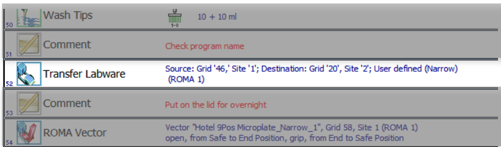
Figure 6. The RoMa "Transfer Labware" command is highlighted, as seen in the Script Editor window.
