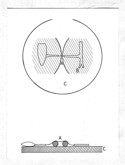
Figure 6. Air Gep Constructed on a Glass Plate.
