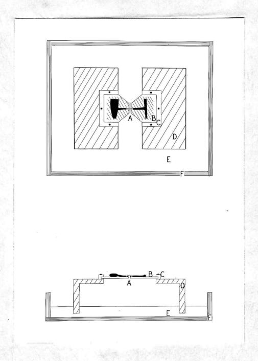
Figure 7. Air Gap Between Two Unconnected Plates.
