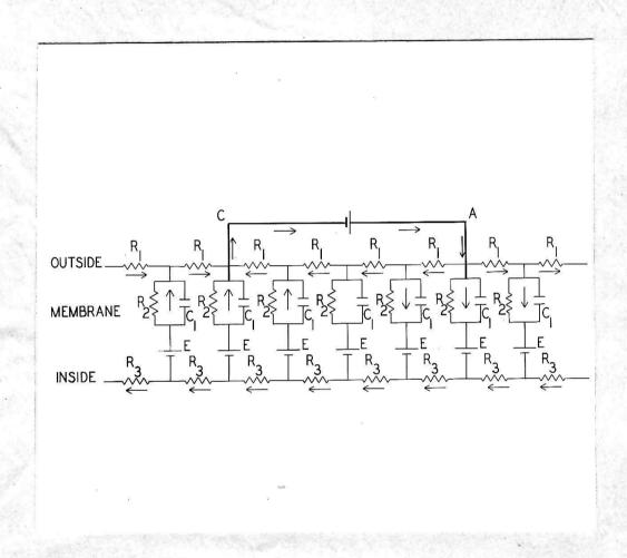
Figure 1. The Equivalent Electrical Circuit of the Nerve Membrane. Modified after Fulton (19).
