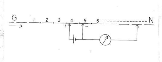
Figure 3. Anodic and Cathodic Polarization of Adjacent Ranvier Nodes. Modified after Blair & Erlanger (24).
