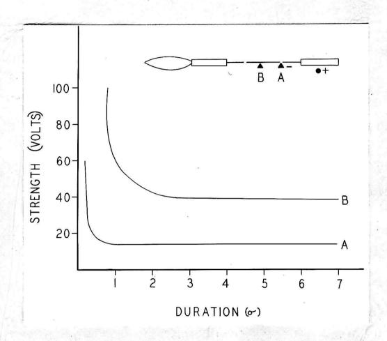
Figure 4. Strength-Duration Curves for a Single Medullated Nerve Fiber. After Kato (26).
