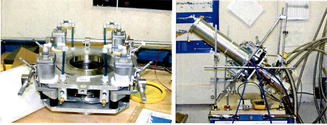
Figure 3.6: Left: pneumatic vibration isolator; Right: mechanical cryocooler operating at a 45^\circ – vibration isolator is designed to comply with tilt in a single direction.
