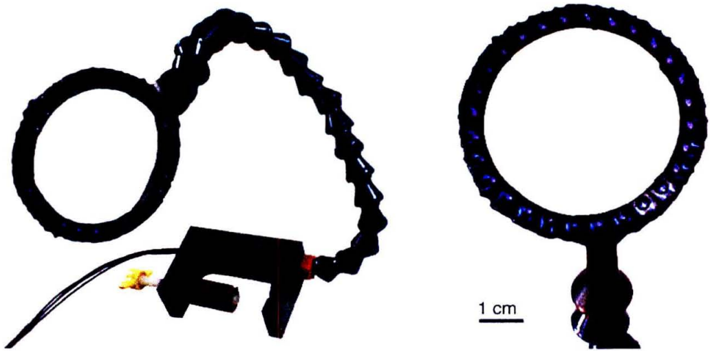
Figure A.14 Ring arrangement of infrared LED's for homogeneous illumination
