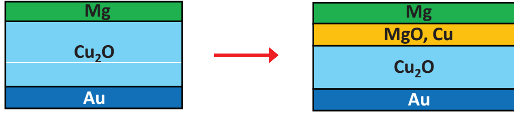
Figure 6.1. Schematic of Cu precipitation in \text{Cu}_2\text{O} solar cells showing the reaction of a metal, in this case Mg, with \text{Cu}_2\text{O} to yield metal oxide and elemental Cu. The interfacial Cu formation reaction limits solar cells based on \text{Cu}_2\text{O} absorbers by transforming them into low barrier height Cu/ \text{Cu}_2\text{O} Schottky diodes.
