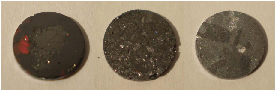
Figure 2.8. Images of diced wafers of (left) mixed-phase \alpha -ZnP 2 , \beta -ZnP 2 , and \alpha -Zn 3 P 2 , (center) \alpha -Zn 3 P 2 with a high density of voids, and (right) large-grain polycrystalline \alpha -Zn 3 P 2 . The displayed wafers have diameters of 1 cm.
