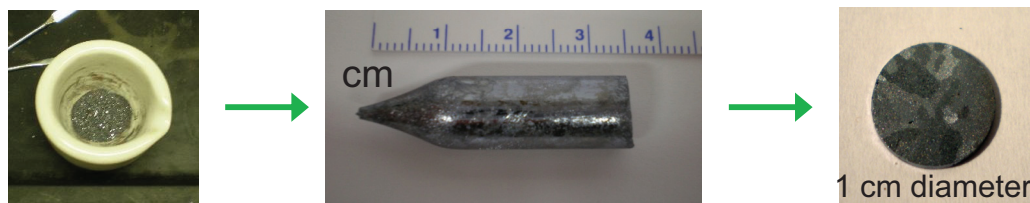
Figure 2.1. Images of the products in the crystal growth process of (left) raw \text{Zn}_3\text{P}_2 crystals, (center) large-grain polycrystalline boule of \text{Zn}_3\text{P}_2 , and (right) diced \text{Zn}_3\text{P}_2 wafer.
