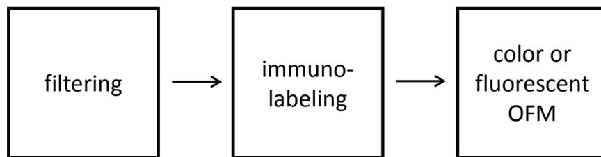
**Figure 6.2.1** A flow chart of a method to detect microbial cells in a water sample
