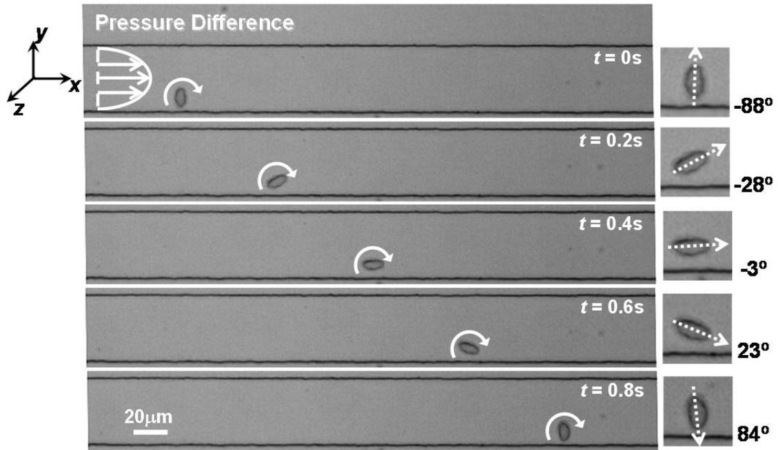
**Figure 2.2.1** An experimental illustration of the microfluidic motion of a *Giardia* cyst driven by pressure difference
