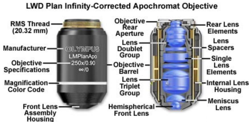
**Figure 1.1.2.2** A schematic of a microscope objective
