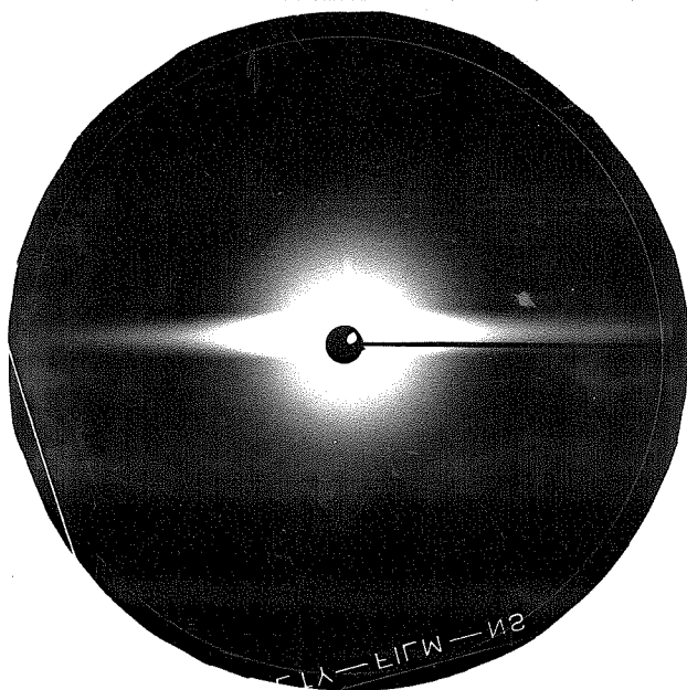
Fig. 21. X-ray scattering patterns of bovine serum albumin on Kodak Medical No-Screen film at a sample-to-film distance of 48 cm. The upper exposure is of a 15% solution for 48.3 hours. The lower exposure is of a 5% solution for 70 hours. Enlarged 1.5 times.
