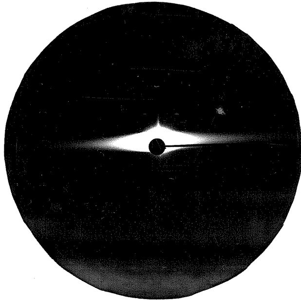
Fig. 22. X-ray scattering patterns of bovine serum albumin on Kodak Medical No-Screen film at a sample-to-film distance of 48 cm. The upper exposure is of 1% solution for 100 hours. The lower exposure is of a background with water for 48.3 hours. Enlarged 1.5 times.
