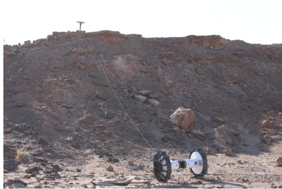
Figure 6.8: *Axel 2* successfully descended a 15 m slope with inclines between  $25^\circ$  and  $45^\circ$  on the first day of testing in Arizona.
