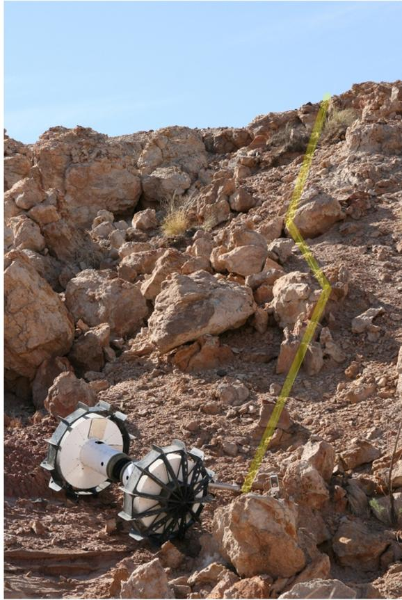
Figure 6.10: *Axel 2*'s tether becomes snagged easily in the field on rocky terrain. The tether is highlighted for clarity. The rover ascended successfully during this test under teleoperation. Future work should use the algorithm developed in Section 4.5 to navigate autonomously in these scenarios and return to the anchor point.
