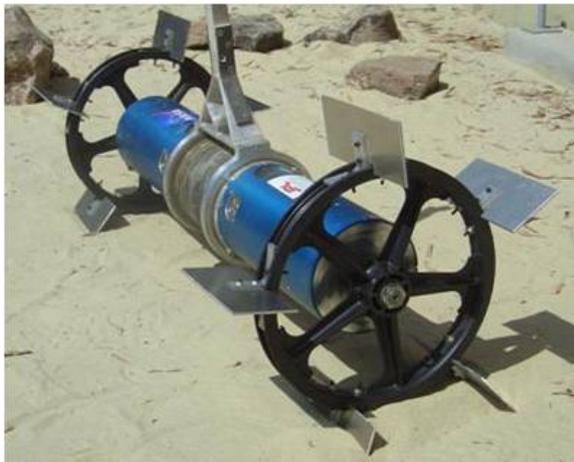
Figure 3.2: *Axel* with 5-grouser wheel design
