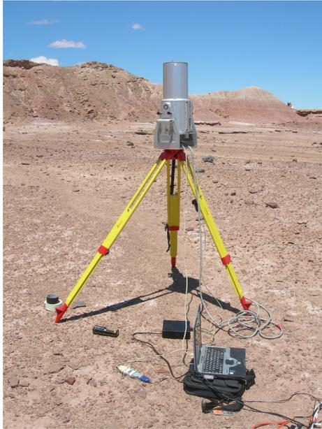
Figure 6.11: Picture of the Riegl 3D laser scanner used to scan terrain in Arizona
