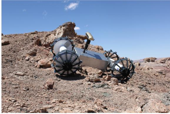
Figure 6.7: *DuAxel* at a Mars analogue site in Arizona climbing up a terrain with slope angles up to  $35^\circ$
