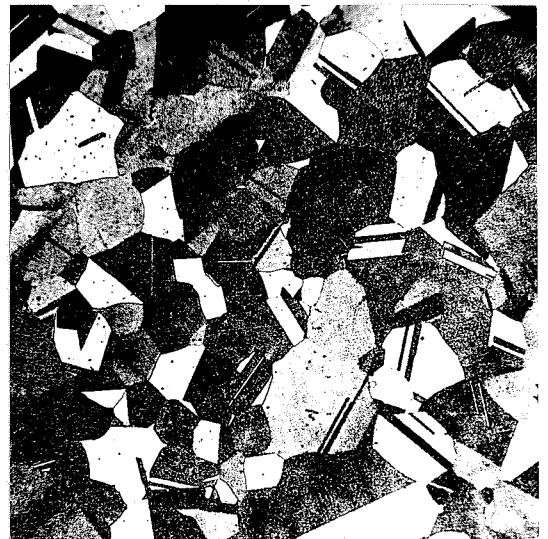
Fig. 5.--91.9 Atomic Pct Au. Heat-treated at 1000°C for 30 minutes and water quenched. Etched. 250X.
