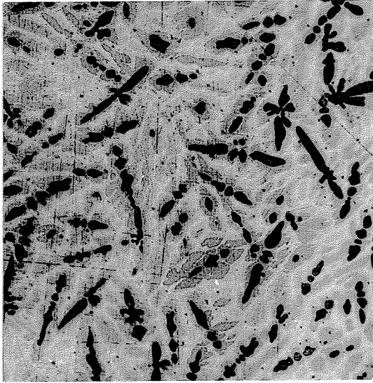
Fig. 2.--82 Atomic Pct Au. As cast. Etched lightly. 250X.
