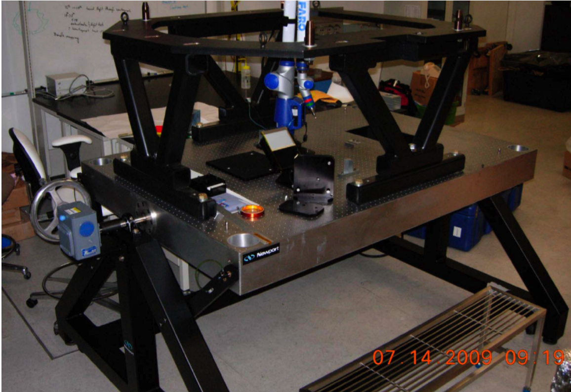
Figure 2.40. The CWI optical bench installed on the rotating structure. Attached to the breadboard is the mounting structure that connects the instrument to the telescope. This consists of three square 3" tubes bolted to the bench, serving as reinforcement and a mounting point for the welded structure above it. A 1" thick steel top plate is a rigid platform for four specially notched interface pins that insert into the telescope Cassegrain ring. Welded to this plate are three triangular legs that are rested on the aforementioned bars. A FARO arm that was used for positioning some of the elements is seen mounted to the bench.
