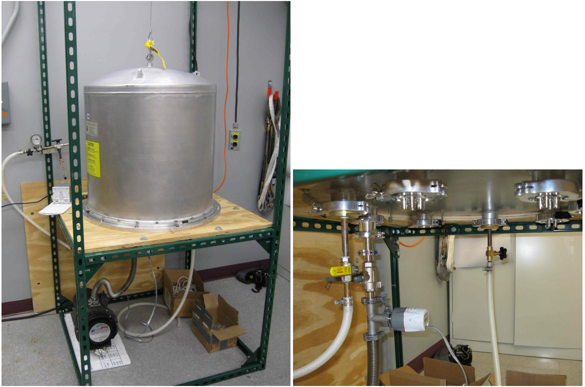
Figure 10.18: Top: Picture of ProtoCage aluminum bell jar on its stand. Bottom: Picture of the bottom of the bell jar's baseplate showing NW40 ports for SHV and gas connections.
