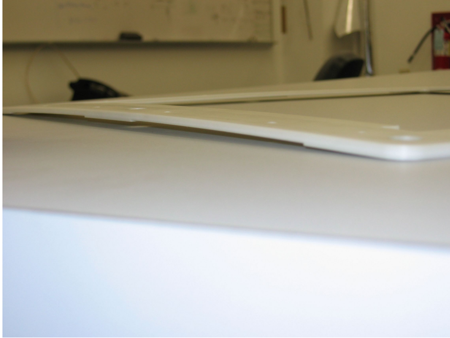
Figure 10.7: “Potato chip” bowing of Delrin frame over time.
