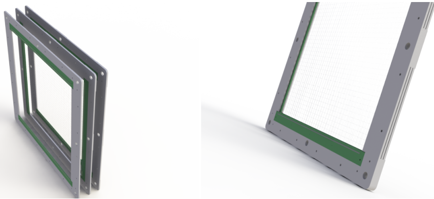
Figure 10.1: Left: CAD rendering of three wire planes mounted on plastic frames. Right: CAD rendering of MWPC unit formed by mating three wire planes.
