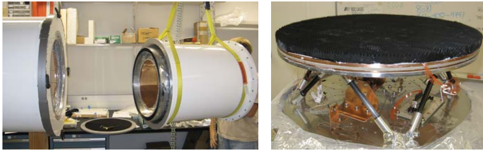
Figure 4.14: Left : The cold load cryostat, about to be bolted to the front of the primary test cryostat. Infrared filters are seen here in both the test cryostat and the cold load cryostat. Right : Behind the filters, the cold load cryostat contains a temperature controlled beam filling black body comprised of black Thomas Keating tiles. Small pyramids on the surface increase the number of light scatterings.
