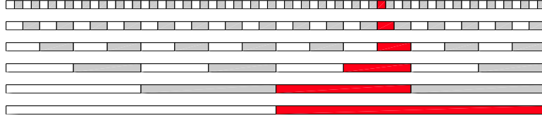
Figure 1.8: Group testing. Suppose N soldiers are tested for a disease using a sensitive but expensive blood test; if blood from different soldiers is grouped together, the test is sensitive enough to declare a “positive” if any of the contributed blood samples were positive. If k soldiers are infected, how many measurements M are necessary? If k is large, then M = N is the best we can do. If k = 1 (and k is known a priori ), then M = \log_2(N) is possible (with or without adaptive measurements). The key idea is to take global measurements and then use reasoning. In this pictorial example, soldier # 45 tests positive, and 45 is 101101 in binary, so using the binary tests depicted by the gray shading, and assuming k = 1 , we can deduce that this is the infected soldier. Each row represents one test, which involves the columns that are gray. See [GS06a] for more info. This was first proposed in the 1940s by two economists helping the military screen draftees for syphilis; their proposal was to group together the blood of five men and apply the test. Since few men were likely to have syphilis, this saves tests on average. The test was never put into practice, in part because the test was barely sensitive enough to detect a positive hit from diluted blood. The subject was revived again in the late 1950s.
