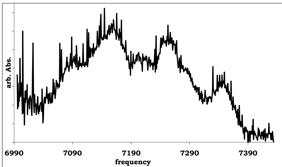
Figure 4.6. CRD spectrum of 2-butene in the 7000 - 7400 \text{cm}^{-1} region. The absorption features are flat after 7390 \text{cm}^{-1} .
