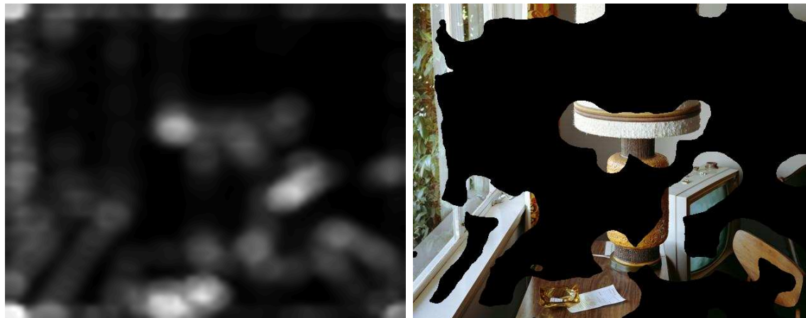
Figure 10.1: The spectral residual saliency map (left) results in candidate object regions (right) when thresholded.
