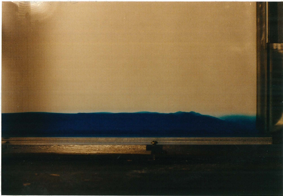
Figure 4.4: Flooded internal hydraulic jump. Approximately 50 cm of channel.
