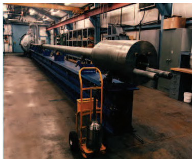
(a) Powder gun located at the STAR facility
