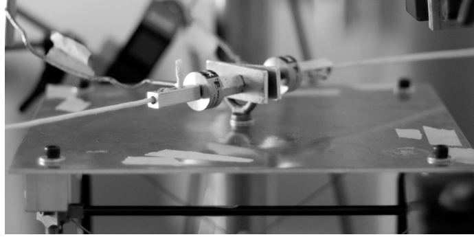
Figure 4.6: Detail of force sensors.
