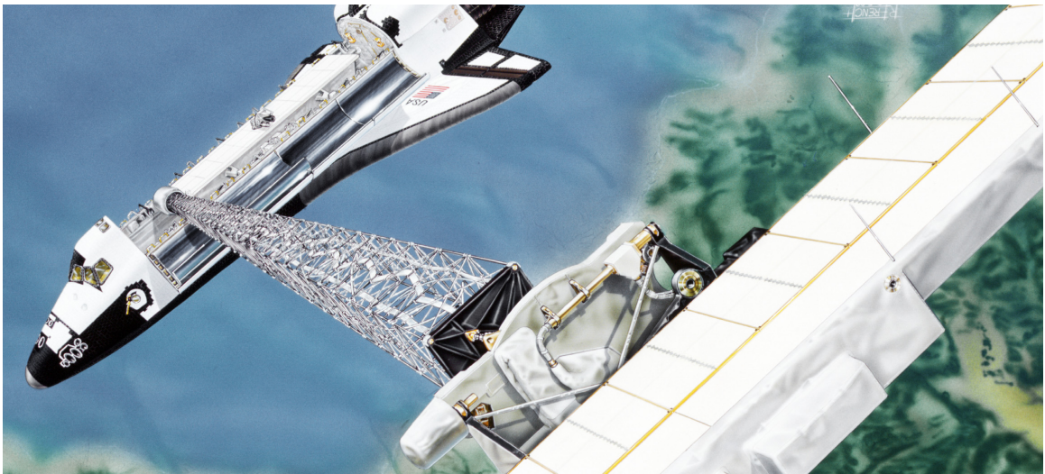
Figure 1.1: Artist's depiction of the Shuttle Radar Topography mission above the earth (NASA image [33]). A mast was used to deploy and stabilize the outboard antenna (foreground) at a distance of 60 m from the orbiter.
