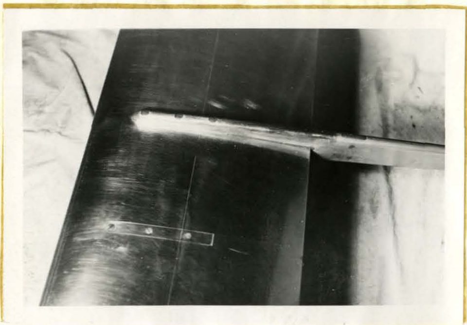
Photo No. 12. Closeup view showing sting attached to wing.
