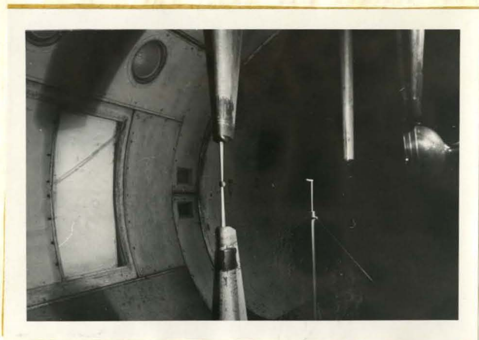
Photo No. 6. Downstream view of all three main windshields and south image wing windshield with bayonets.
