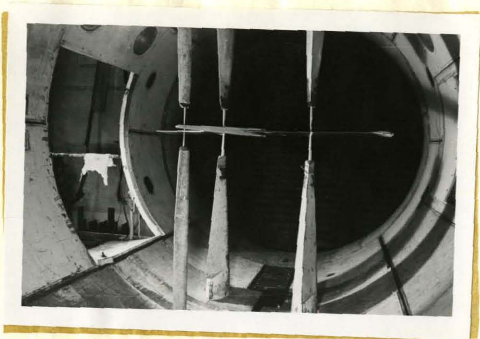
Photo No. 9. View looking upstream showing wing tare setup \psi = 27^\circ .
