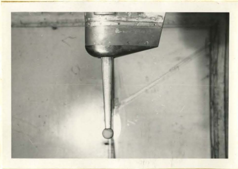
Photo No. 4. View looking across tunnel showing main wing windshield and bayonet with ball tip.
