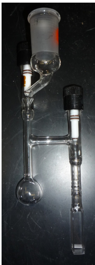
Figure 3.4. Special cuvette used for Hemochromagen Assay, showing the bulb on the left and the quartz cuvette on the right.
