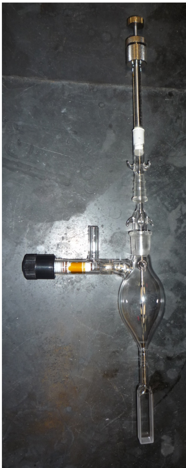
Figure 3.5. Apparatus for chemical redox titration. The protein sample is held in the quartz cuvette at the bottom, the oxidant/reductant is held in the gas-tight syringe above the cuvette. Samples can be degassed and assembled in an anaerobic chamber or degassed on a Schlenk line using the side arm (left).
