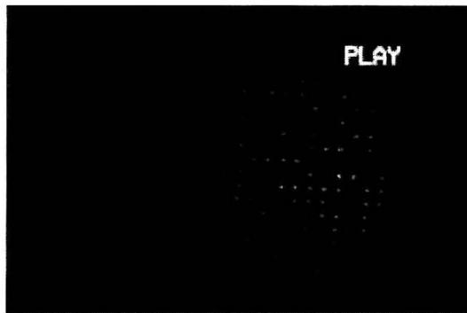
Fig. 6-11. Image rendered by the hologram on the CCD of an  $11\ \mu\text{m}$  pixel mask when illuminated with a white light lamp.
