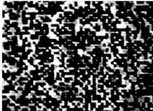
Fig. 3-5. Hologram of a 34  $\mu\text{m}$  pixel-size mask recorded on 100  $\mu\text{m}$  thick Du Pont photopolymer using VCSELs.
