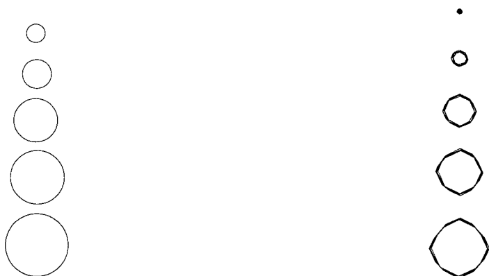
Figure 6.5: Simulation of fast plane rate calibration pattern. (A) Mask, (B) Simulation results.
