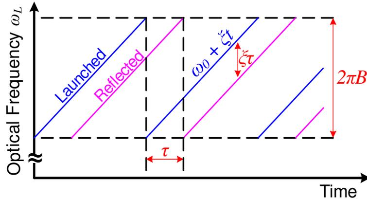
Figure 1.2. A frequency-modulated continuous wave (FMCW) experiment.
