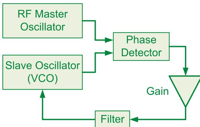
Figure 1.1. Schematic diagram of a generic phase-locked loop.
