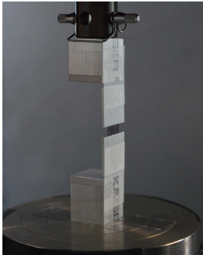
Figure 3.21: Moment-curvature experimental setup
