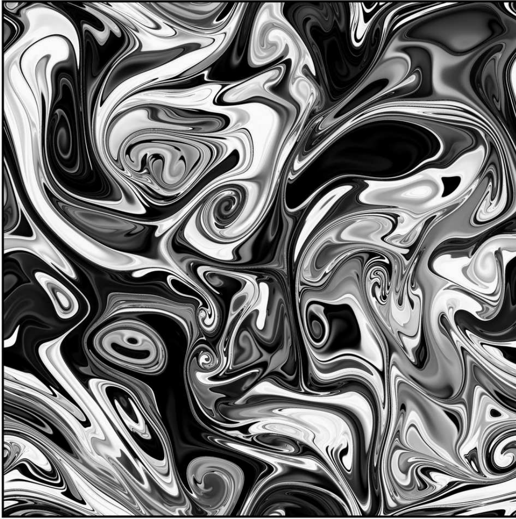
(a) Plane-cut of the full three-dimensional scalar field with resolution 4096^2 , 0 \leq x \leq 2\pi and 0 \leq y \leq 2\pi .
