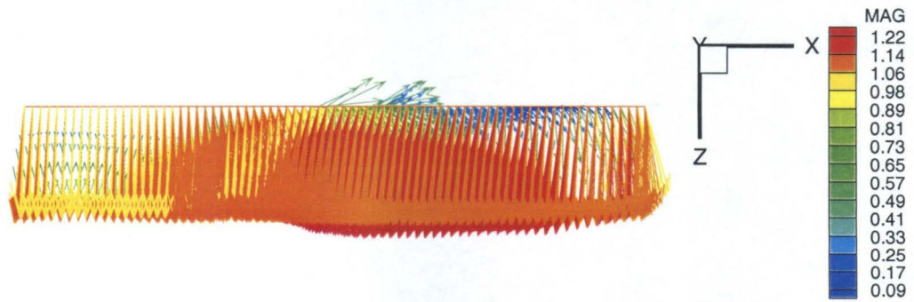
Figure 5.42. 50^\circ wing, \alpha = 7.5^\circ , mean velocity field, top view
