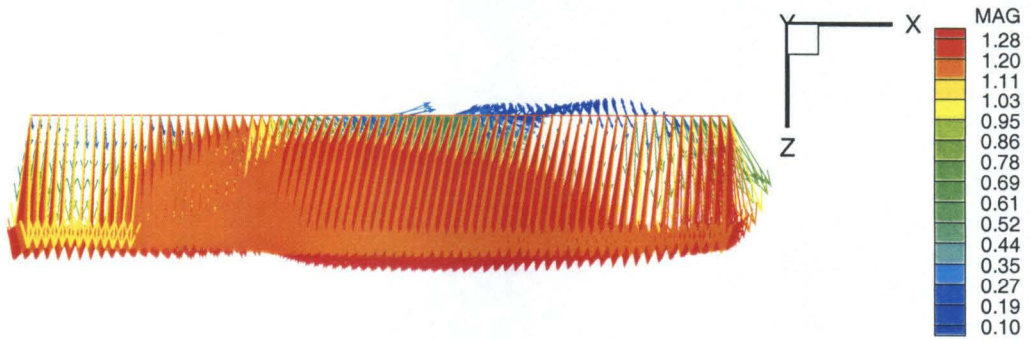
Figure 5.52. 50° wing, \alpha = 12.5^\circ , mean velocity field, top view
