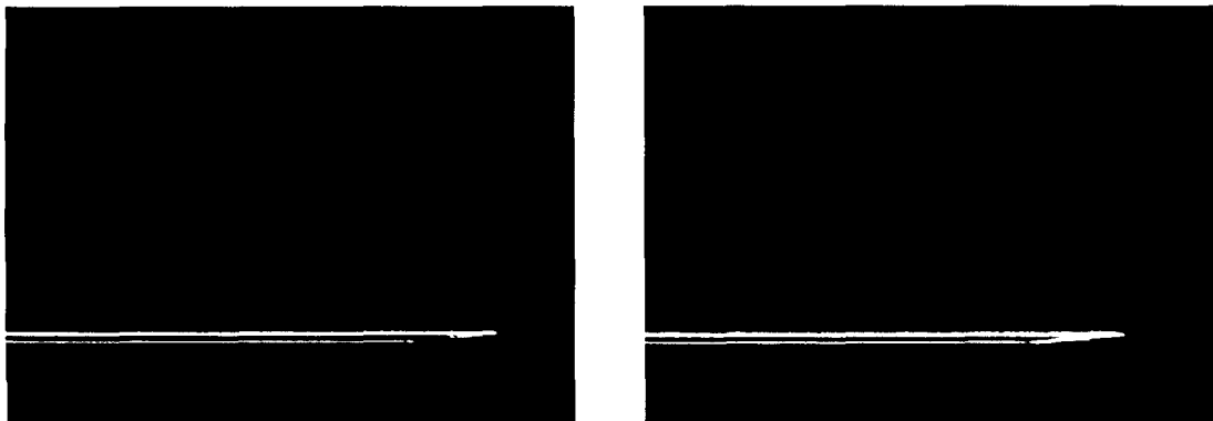
Figure 5.3. 65^\circ wing, \alpha=5^\circ ; typical left and right camera views (dewarped)
