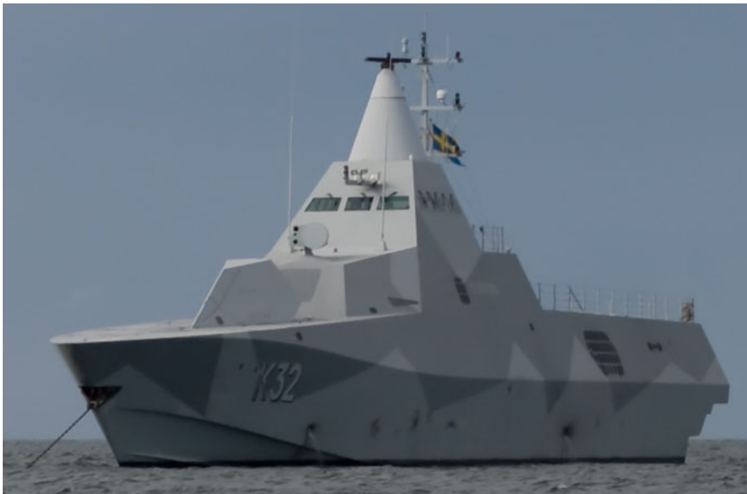
Figure 1.4: Swedish HMS Helsingborg: its hull is constructed with a sandwich design consisting of a PVC core and vinyl external faces reinforced with carbon fibers (figure source: Wikimedia Commons).
