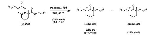
Scheme 3.2 Double asymmetric catalytic alkylation of an enol carbonate ester substrate
