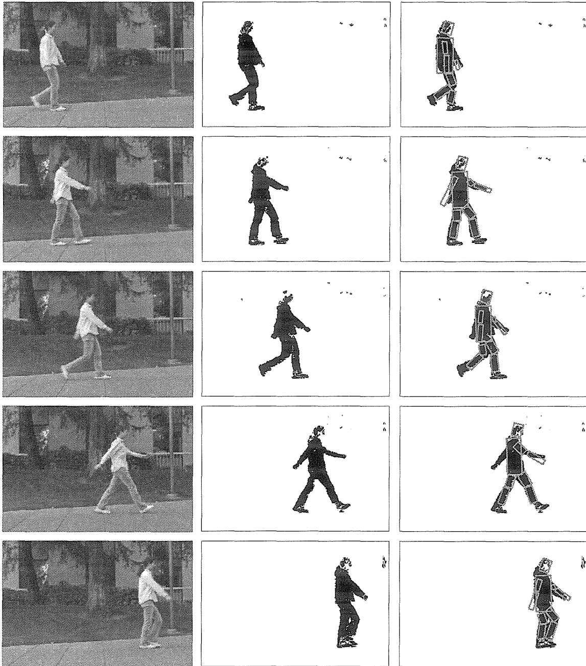
Figure 6.21: A Female Subject Walks from Left to Right. (left): sample images. (middle): foreground data after background subtraction. (right): best fitting codewords.
