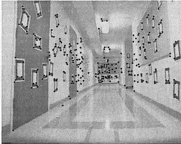
Figure 3.9: Sample Image in the Real Corridor Sequence. Black dots indicate the features detected on the image.
