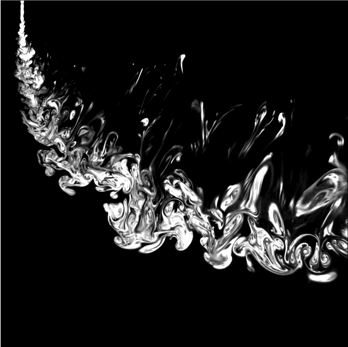
FIG. 2.5 Jet-fluid concentration in a streamwise slice of the jet for Re_j = 1.0 \times 10^3 and V_r \simeq 32.3 ( cf. Fig. 2.3). Image data scaled by x^{1/2} to compensate for downstream decay (for display purposes only).
