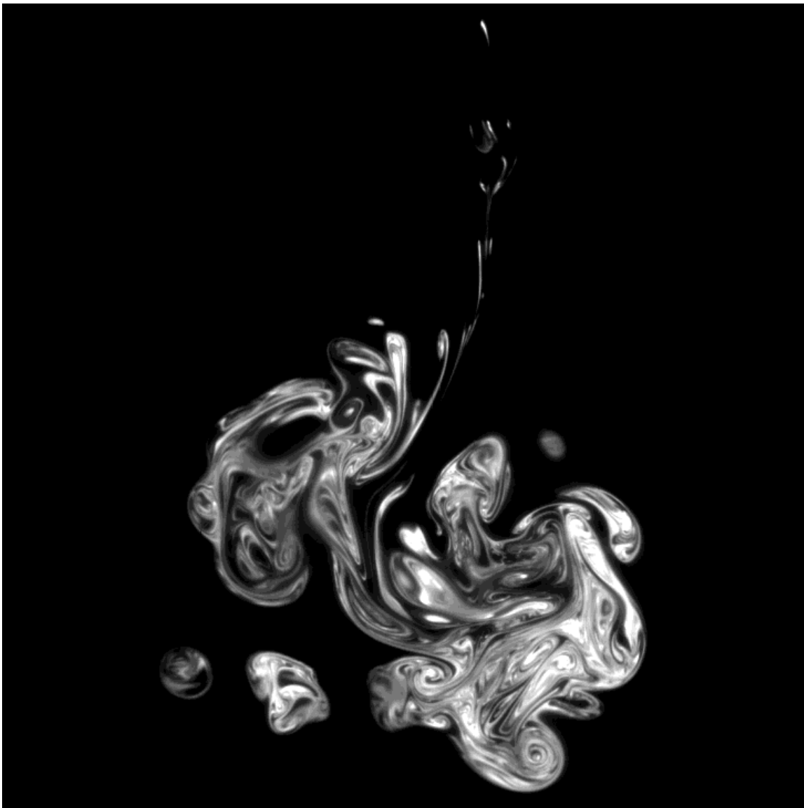
FIG. 2.9 Jet-fluid concentration in a transverse slice of the jet for V_r \simeq 32.3 and Re_j = 1.0 \times 10^3 .
