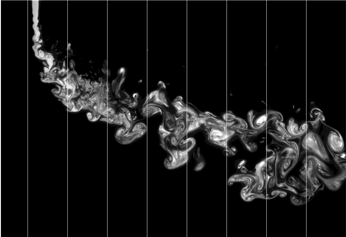
FIG. 4.3 The eight, six-jet-diameter-wide strips used to calculate jet-fluid-concentration PDFs in streamwise sections of transverse jet. The smaller strip at the extreme left does not contain jet fluid, and is not counted as one of the eight, 6d_j -wide strips.
