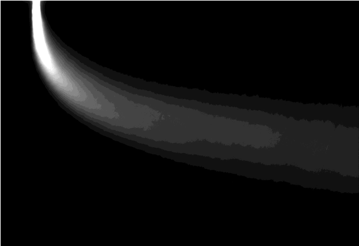
FIG. 3.1 Mean concentration field for Re_j = 10 \times 10^3 and V_r \simeq 10.1 . Ensemble averaged from 254 streamwise (plane-of-symmetry) slices of transverse jet.
