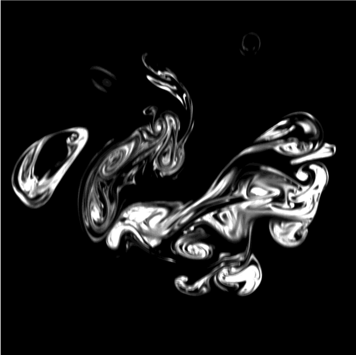
FIG. 2.7 Jet-fluid concentration in a transverse slice of the jet at downstream location x/d_j = 50 . V_r \simeq 10.1 and Re_j = 1.0 \times 10^3 .
