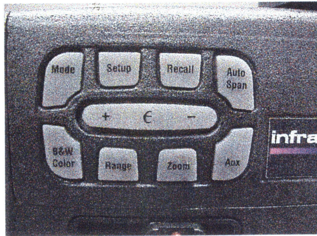
Fig. 4.4. All ThermoCam controls are situated on the main keypad.
