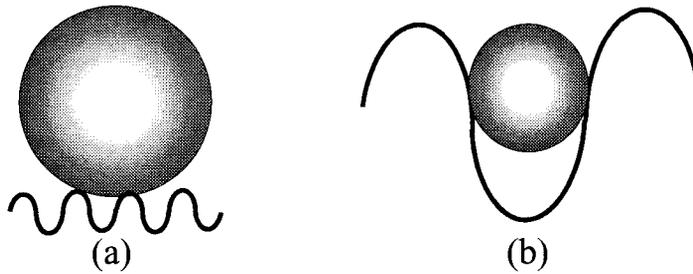
Figure 3-10: Surface roughness effect on particle contact area.
