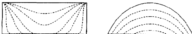
Figure 3.2: Schematic of valve closing for square and rounded channels (77) . The dotted lines indicate the contour of the top of the channel for rectangular (left) and rounded (right) channels as pressure is increased.
