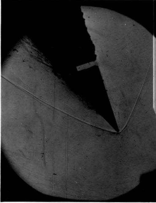
PLATE 19 - FLOW OVER A 44^\circ WEDGE, N_2 - AIR AT P_4/P_1 = 7500 FIGURES INDICATE DELAY TIME IN MICROSECONDS
