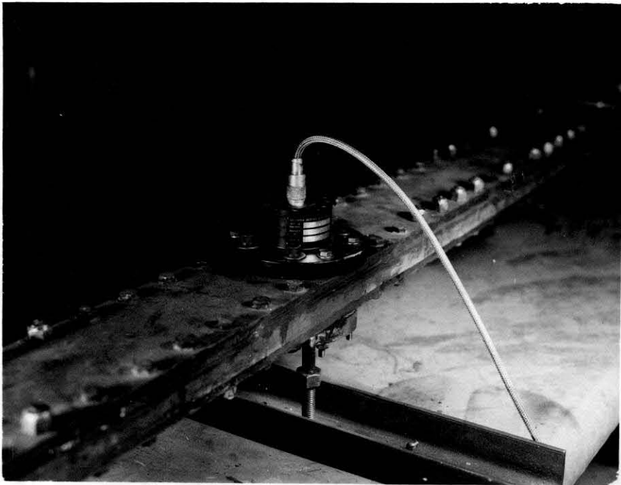
PLATE 5b - QUARTZ PRESSURE PICKUP MOUNTED ON THE UNIFORM EXPANSION TUBE
