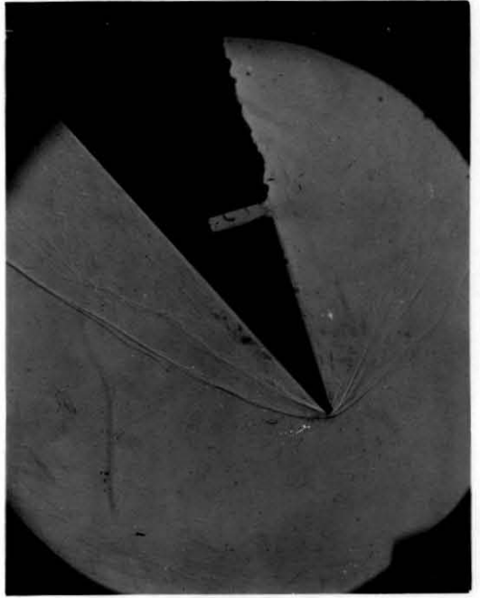
PLATE 19 - FLOW OVER A 44^\circ WEDGE, N_2 - AIR AT P_4/P_1 = 7500 FIGURES INDICATE DELAY TIME IN MICROSECONDS
