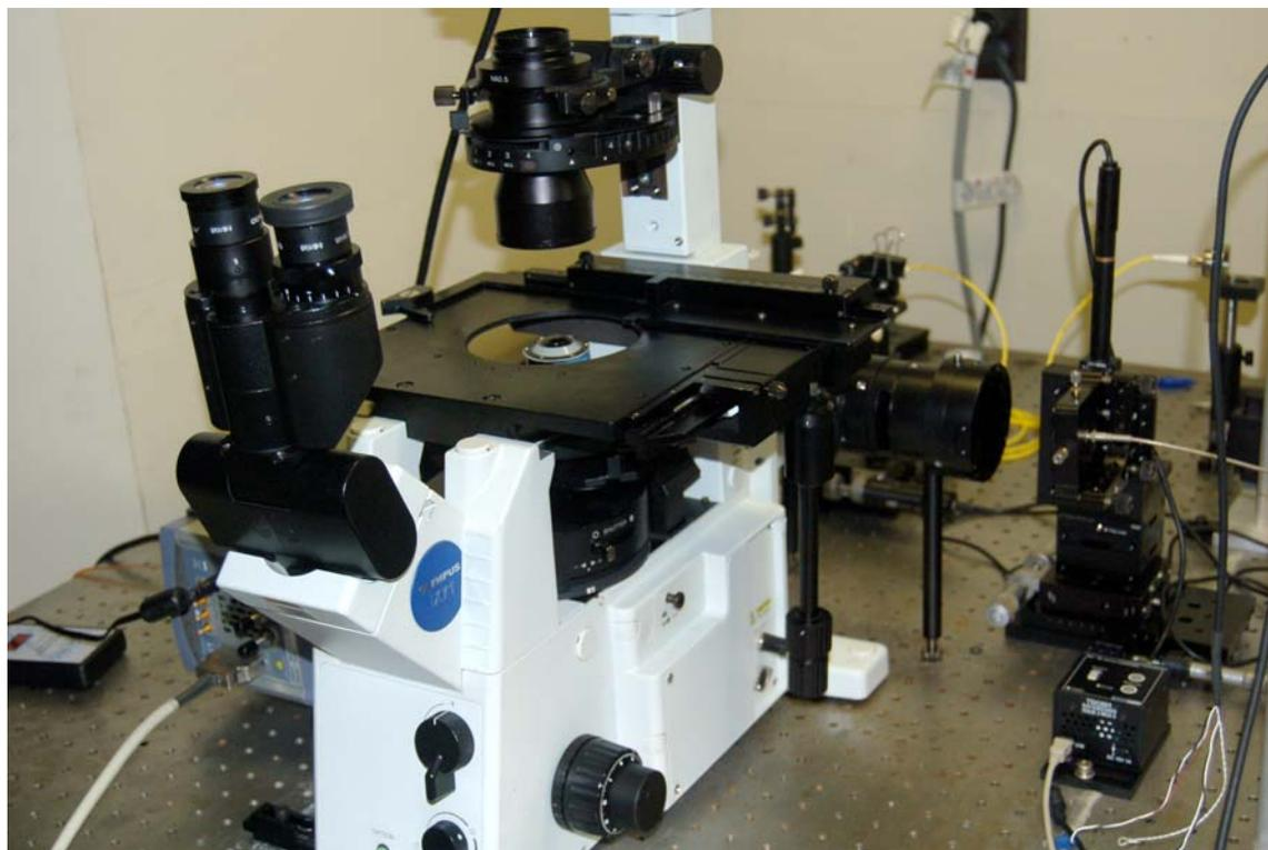
Figure A.11 The complete Olympus IX71 microscope used for the VA-TIRFM study reported in this thesis is shown here. Note the laser positioning assembly on the right.
