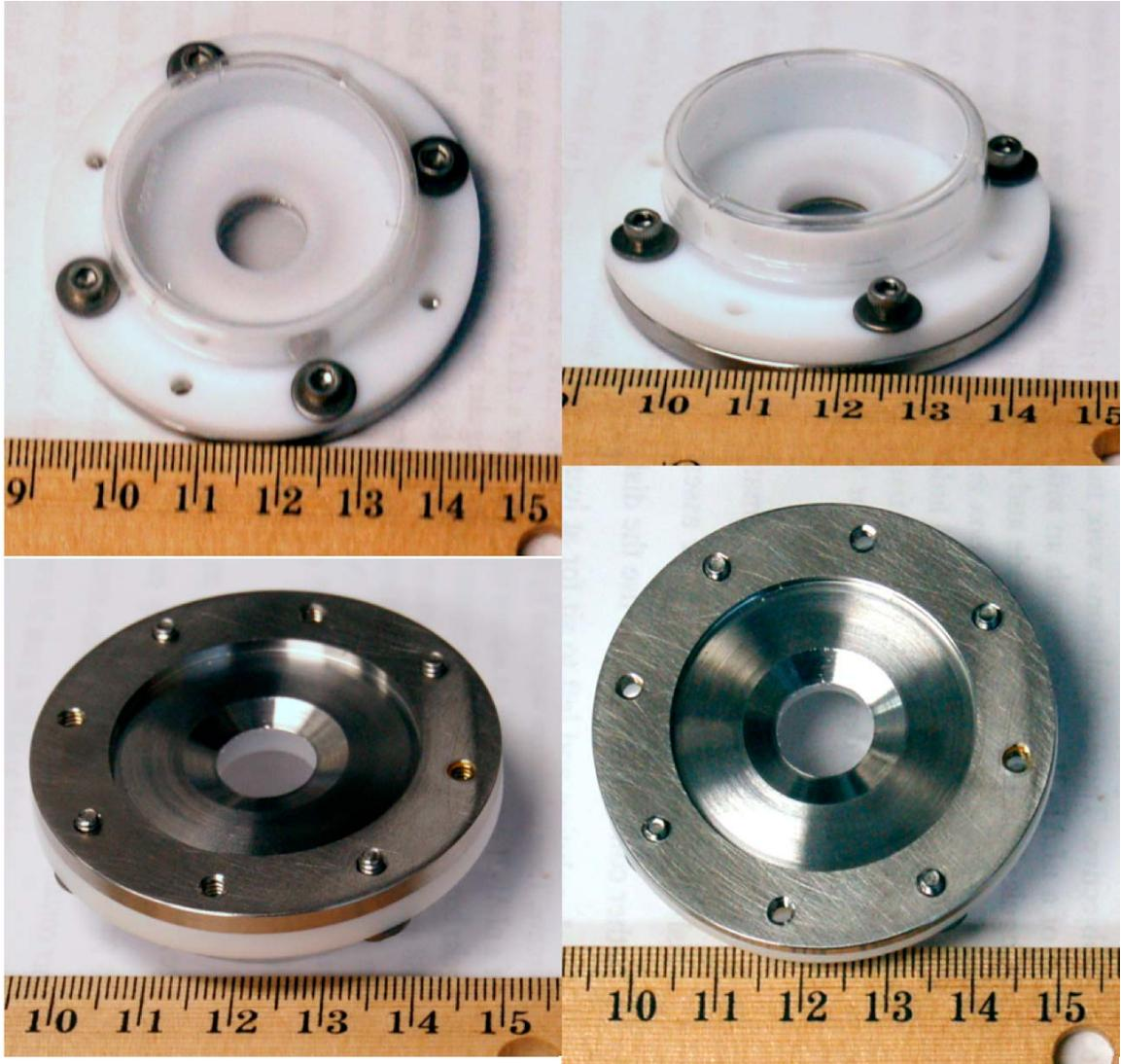
Figure A.10 A fully assembled culture dish is shown above from the top and also from the bottom.
