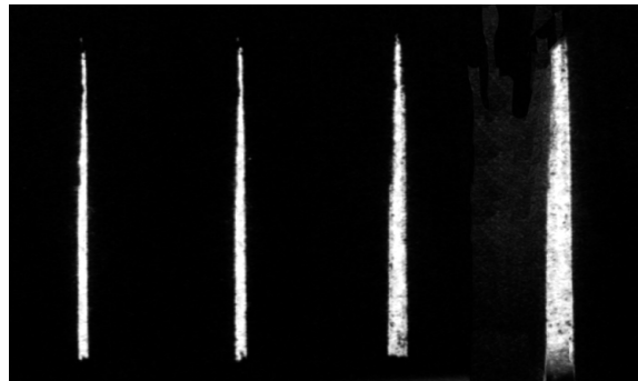
Figure 2.22: CGS fringe patterns at (left to right) 3, 38, 78, and 138 \mu\text{s} for a 6Al-4V Ti specimen impacted at 9 m/s. (Beam diameter = 50 mm)
