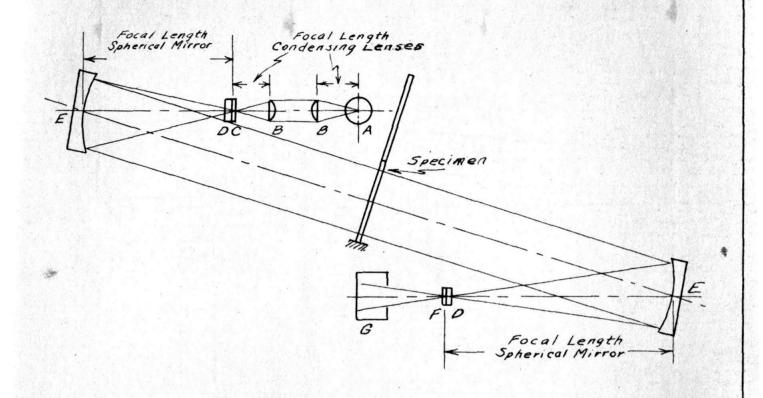
DIAGRAMATIC PLAN OF POLARASCOPE
