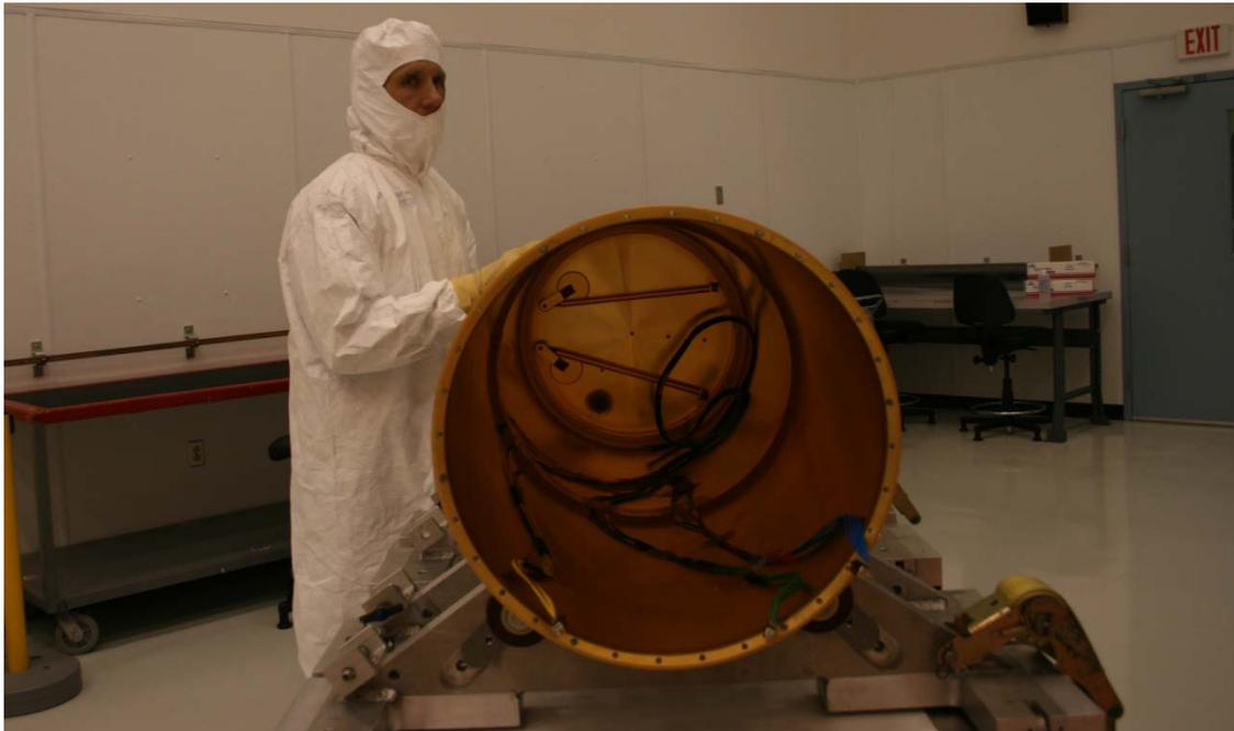
Figure 2.3.1 The CIBER experiment section rocket skin. Cabling for the shutter door runs along the inside of the skin from the forward bulkhead.
