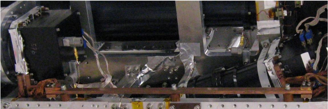
Figure 2.5.6 The NBS thermal bus copper bar.
