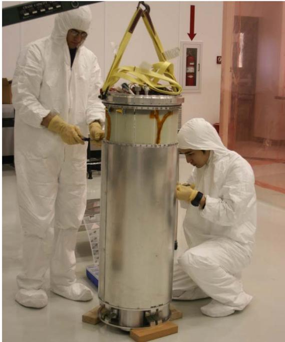
Figure 2.3.7 Installing the radiation shield.
