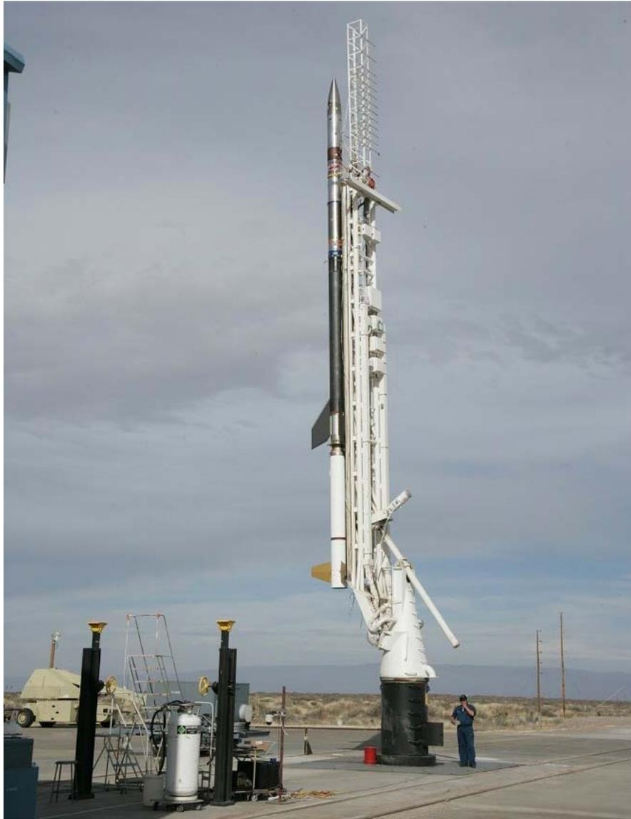
Figure 2.7.6: CIBER on the Athena rail launcher during the range vertical test.
