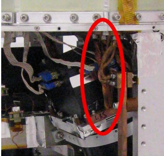
Figure 2.5.5 The LRS and NBS thermal strap copper braids installed in the cryostat.
