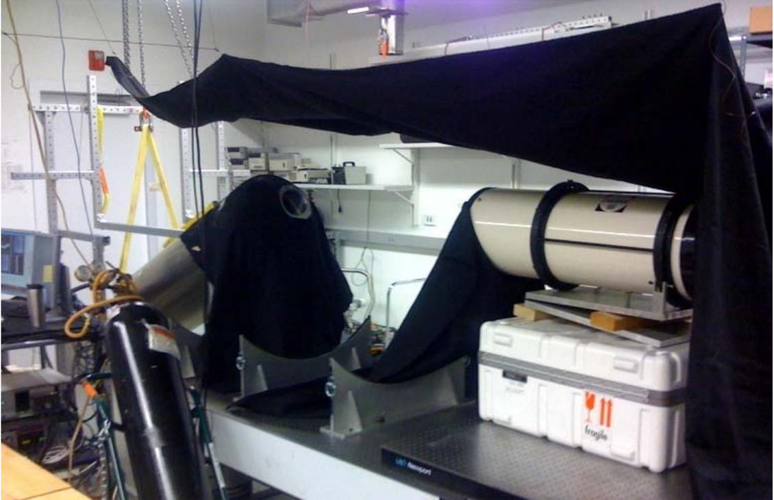
Figure 4.1.3 To map the large-angle rings, the collimator was fixed in position, and the cryostat was rotated up and down by a hoist at the back.
