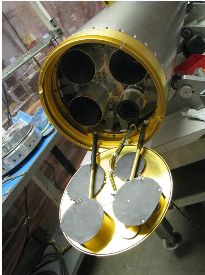
Figure 2.3.3 The CIBER shutter door, open and in the first flight configuration with individual cold plates for each instrument.
