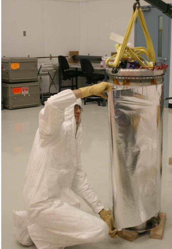
Figure 2.3.8 Wrapping insulation around the radiation shield.
