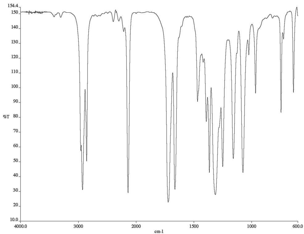
Figure A2.2.18 Infrared spectrum (film/NaCl) of compound **145**
