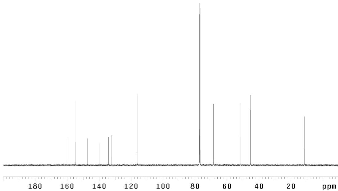
Figure A2.2.6  $^{13}\text{C}$  NMR (125 MHz,  $\text{CDCl}_3$ ) of compound **128**
