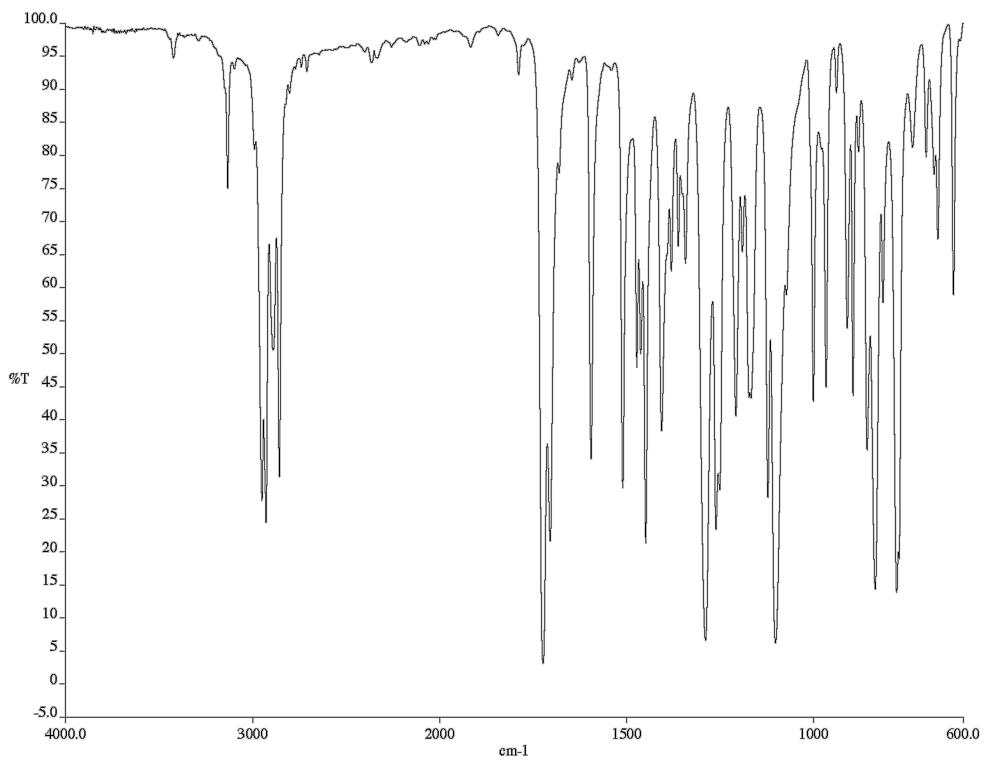
Figure A2.2.2 Infrared spectrum (film/NaCl) of compound **136**
