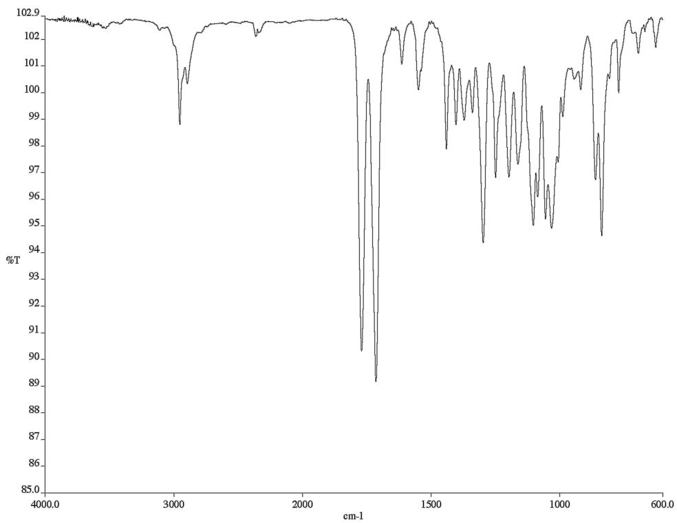
Figure A2.2.79 Infrared spectrum (film/NaCl) of compound **175**
