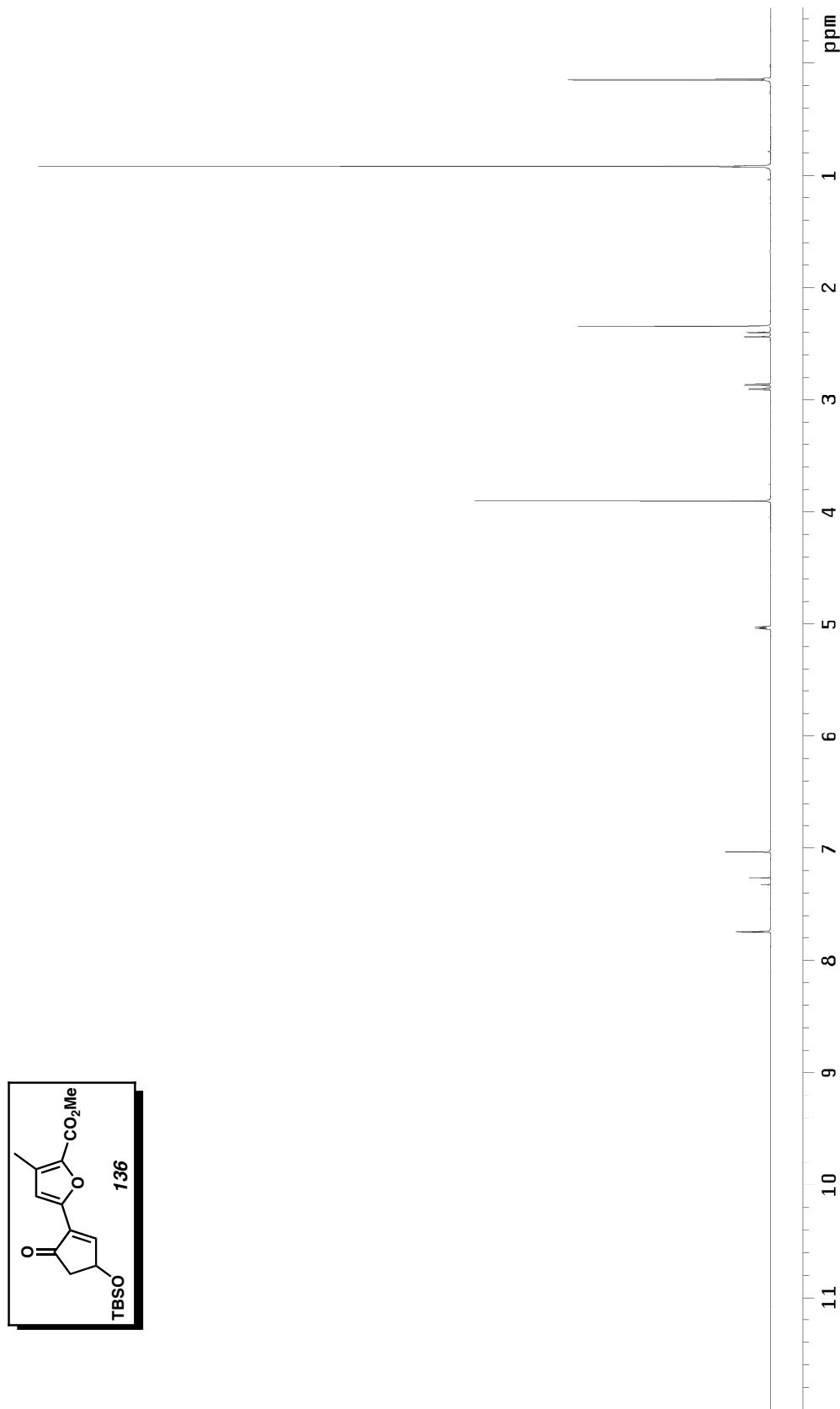
Figure A2.2.1  $^1\text{H}$  NMR (500 MHz,  $\text{CDCl}_3$ ) of compound 136
