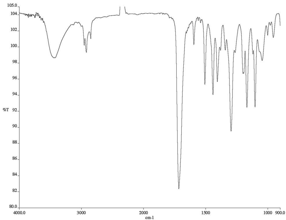
Figure A2.2.5 Infrared spectrum (film/NaCl) of compound **128**
