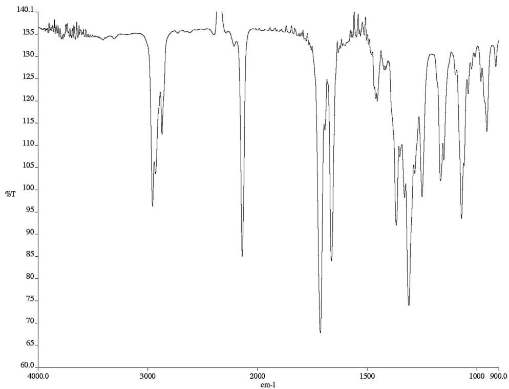
Figure A2.2.21 Infrared spectrum (film/NaCl) of compound **147**
