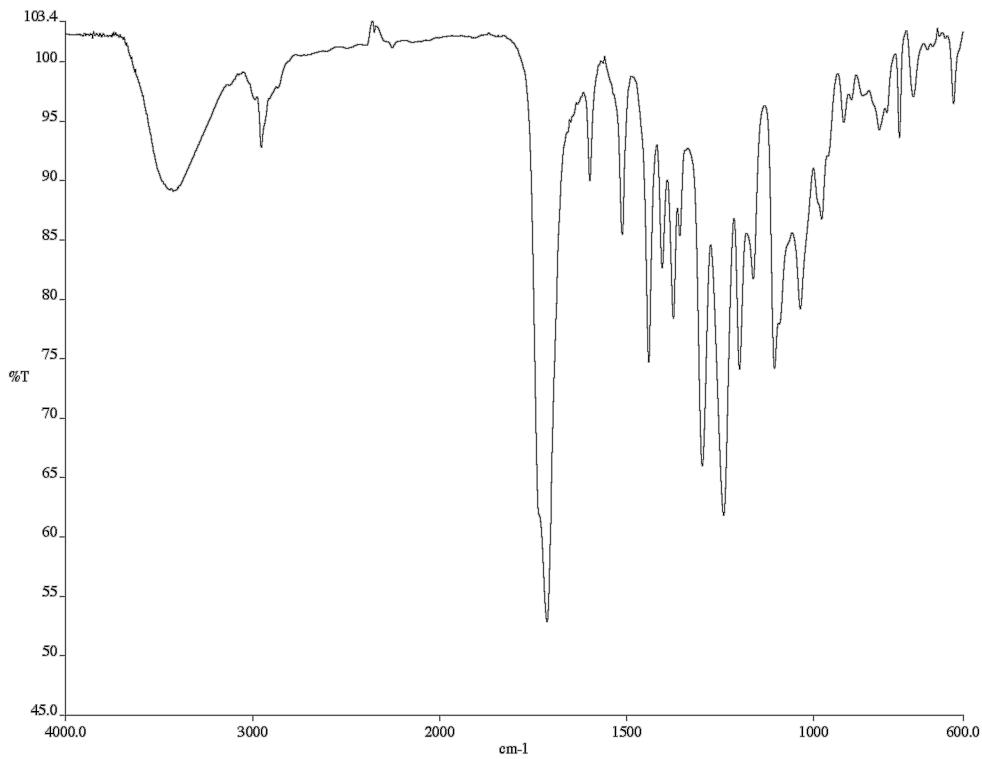
Figure A2.2.52 Infrared spectrum (film/NaCl) of compound **164**
