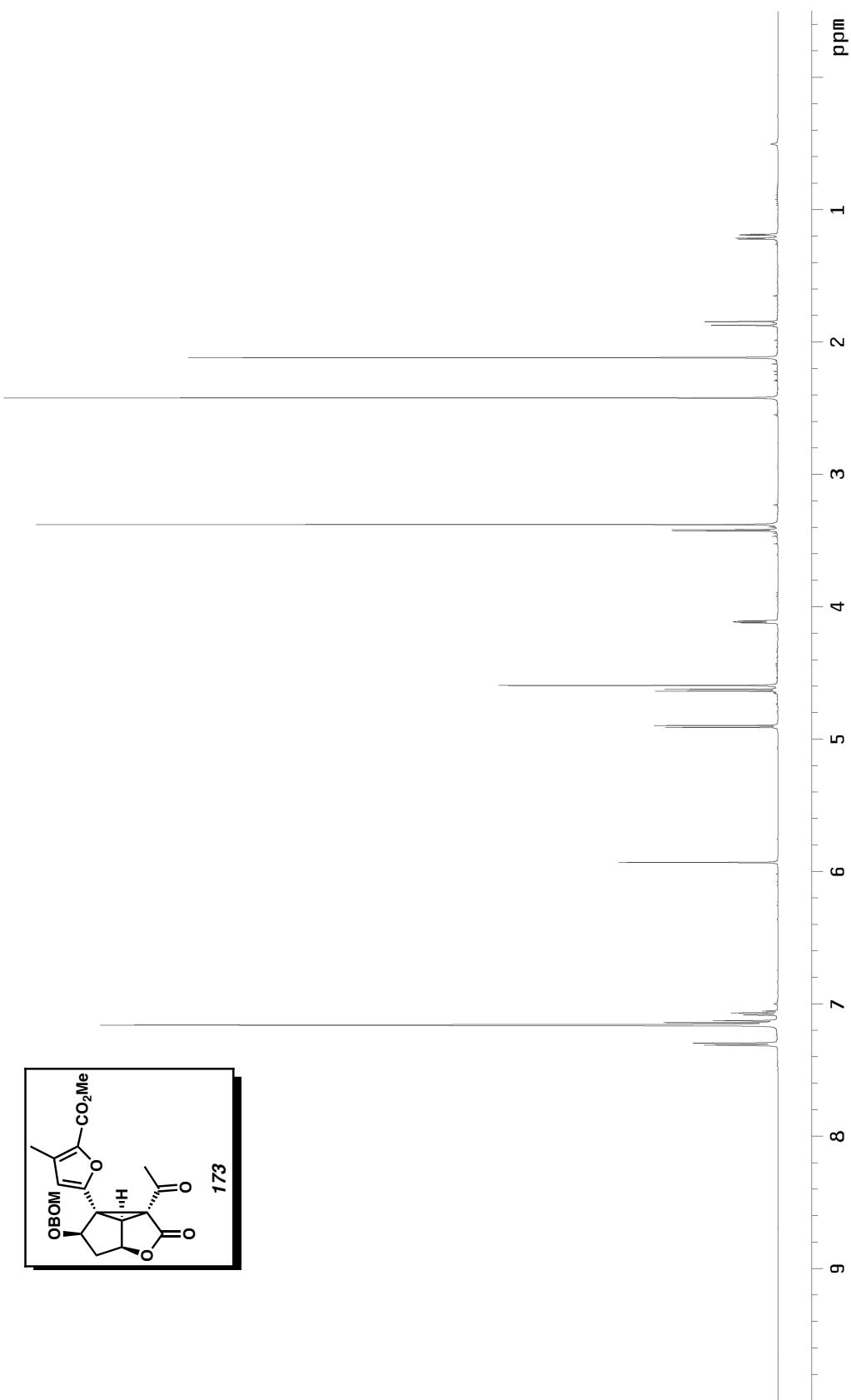
Figure A2.2.72  $^1\text{H}$  NMR (500 MHz,  $\text{C}_6\text{D}_6$ ) of compound 173
