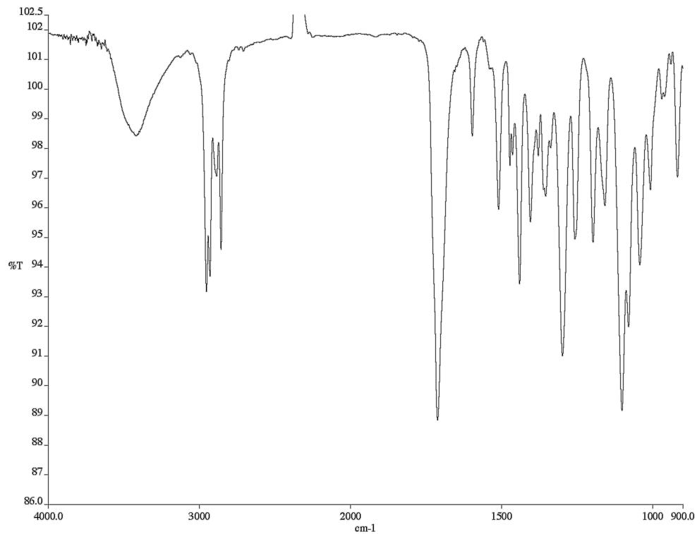
Figure A2.2.49 Infrared spectrum (film/NaCl) of compound **37**
