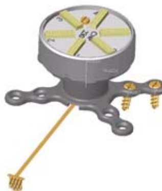
Figure 2.27. Schematic of the packaged silicon probes. The design shows a 96-channel device consisting of three 32-channel devices. The legs of the titanium pedestal are secured to the skull with bone screws.
