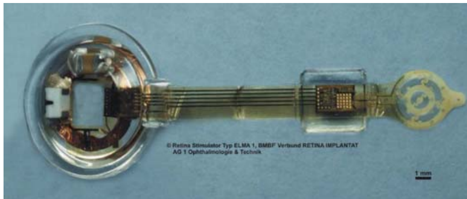
Figure 1.7. Final implant with parylene C and silicone rubber encapsulation [71].
