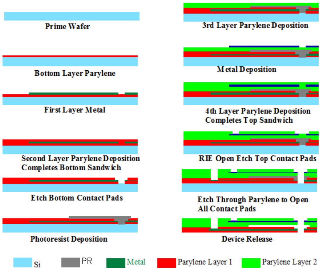
Figure 2.16. Fabrication process for dual layer pocket.
