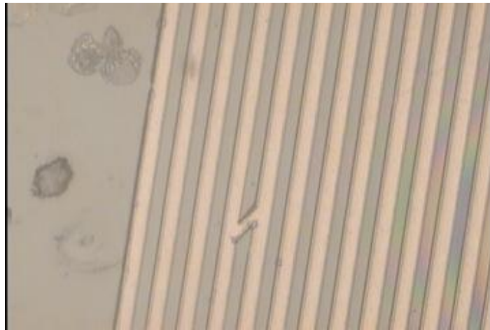
Figure 5.28. Short circuit defect on dense metal lines.
