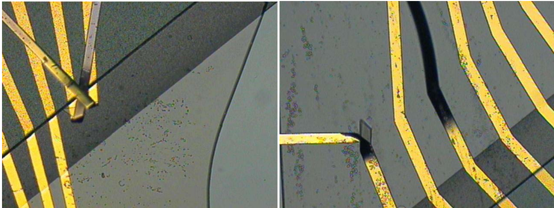
Figure 5.7. Detached gold lines after the underlying chrome has been etched away due to isotropic undercut etching.
