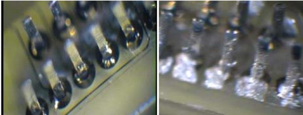
Figure 2.25. Proximal bonding of commercial connector with parylene cable connector pads; (left) before bonding; (right) after bonding with conduction epoxy.
