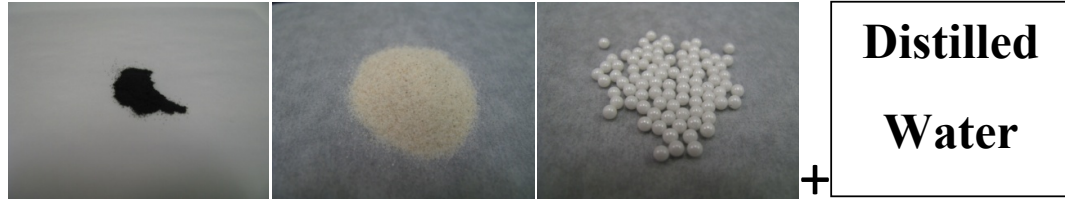
(Pt catalyst: 0.10~0.45 \mu\text{m} ) (Silica: 100~500 \mu\text{m} ) (Zirconia balls, O.D: 1/8 in)
