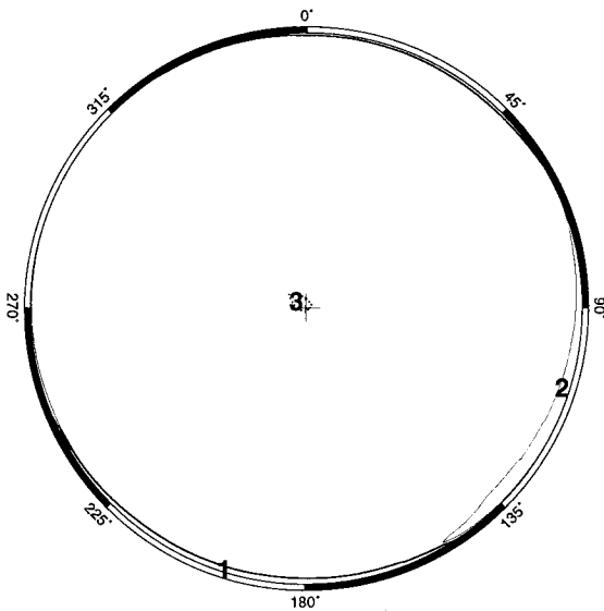
Figure 5.7: Stress inversion results in Cook Inlet, Alaska using all identified breakouts from all available wells excluding the breakouts from wells Gp51 and Smgs6. Plotting conventions are the same as Figure 5.6.
